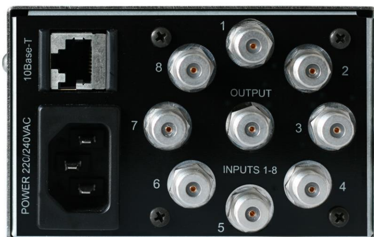
Figure 2 Back panel of 1 switch unit with F connectors
